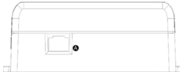
Figure 13 - RF542 RJ45 Network Port
